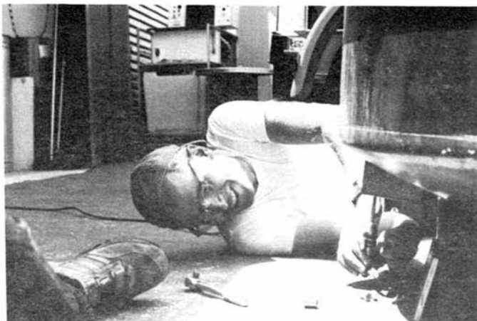
Hugh Hixon preparing to mount the shock absorbers on the dewar feet.
