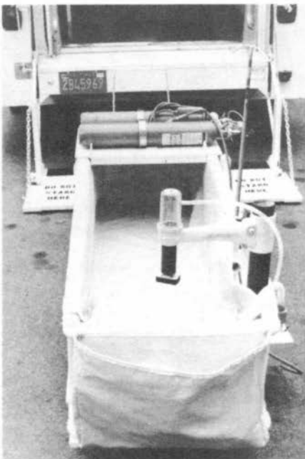
Portable Ice Bath on the end of the ambulance lift gate with portable HLR mounted and O 2 bottles in rack.
