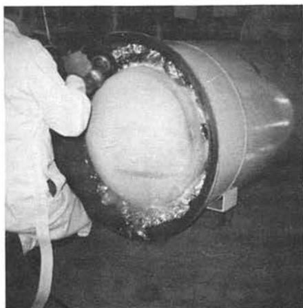
Gallo technician Mogens Friedlow opens the inner cylinder of the Cryo-Care dewar with an abrasive cutting wheel in preparation for moving Dr. Bedford into the Galiso dewar.
