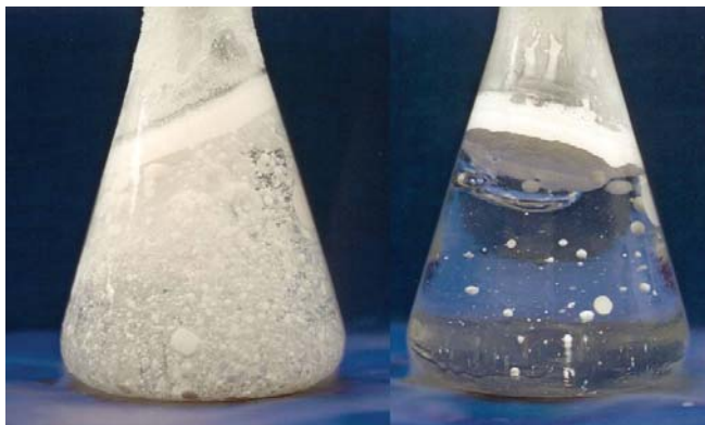
Figure 5. Effect of ice blockers on ice formation. The flask on the left contains 55% w/w ethylene glycol solution that was cooled to -130°C. The flask on the right contains the same solution, except with 1% of the ethylene glycol replaced by 0.9% X-1000 and 0.1% Z-1000 ice blockers. It is almost completely vitrified, with the majority of the solution being a transparent glass rather than white crystalline ice.
